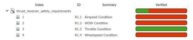
The results show that 3 out of the 4 safety properties are falsified and that one property is valid. The design requirements for the aircraft thrust reverser system do not correctly capture the safety requirements. You must redesign it to validate the safety properties.
