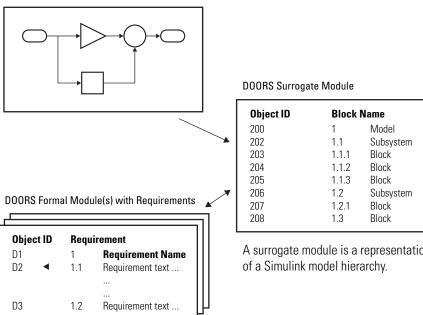
Enter requirements in the DOORS formal module and link them to objects in the DOORS surrogate module, so you can navigate from requirements to Simulink objects.
