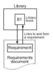
When you use library block B1 in a model, you can navigate from the reference block to the requirement. However, the link from the requirement still points only to library block B1, not to the reference block.
