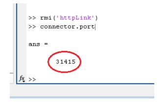
**Update Backlinks** feature requires that HTTP server is activated for port 31415. If connector.port command returns a higher number, this indicates that the desired port number was taken by some other process when this instance of MATLAB was started. You will need to:
