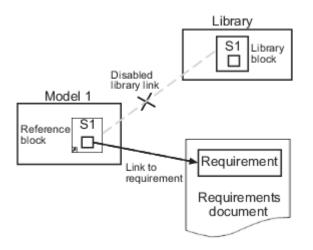
**Note** When linking to a requirement from inside a reference block, you can create links only in one direction: from the model to the requirements document. The RMI does not support inserting navigation objects into requirements documents for objects inside reference blocks.
